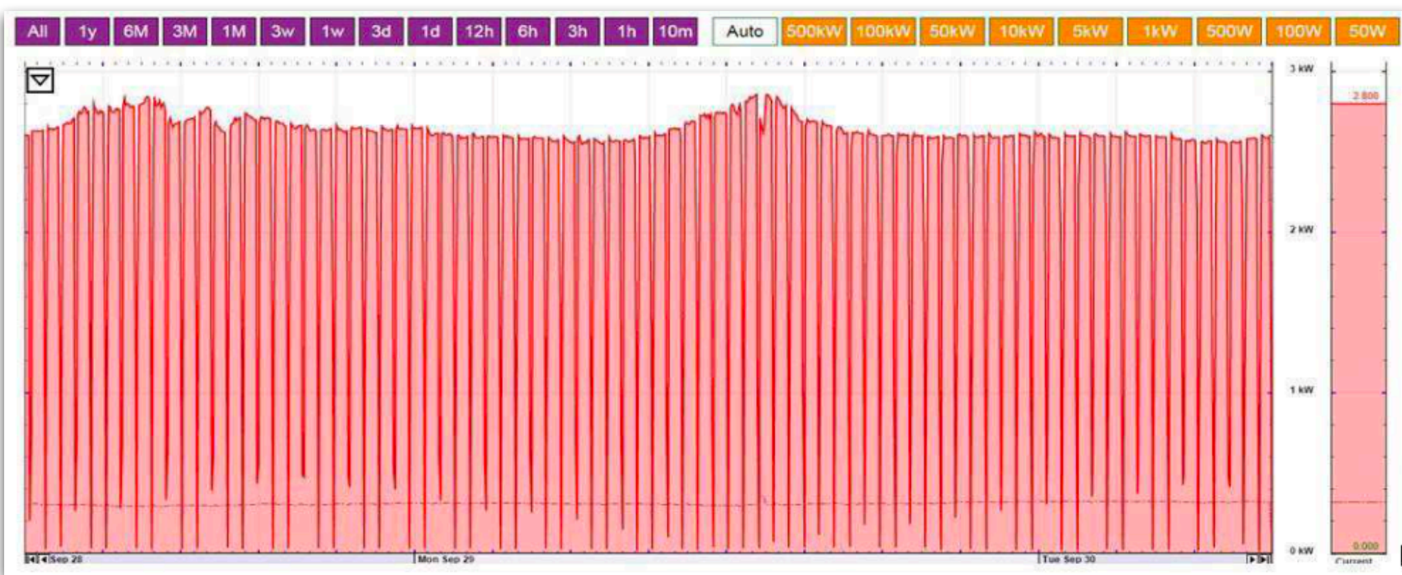
Power Usage for Sample “A” test for 48 Hours at 65°F set point
