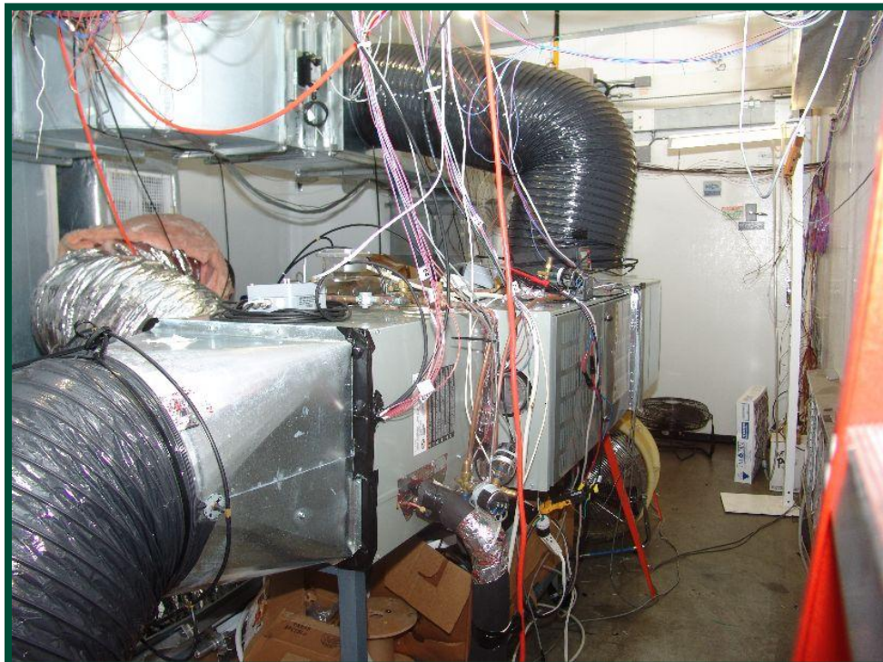
FIGURE 2. PICTURE OF THE INDOOR SECTION OF THE AIR-CONDITIONING UNIT IN THE INDOOR TEST CHAMBER
